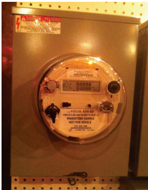
Figure D-1 FOCUS AXR-SD Silver Spring Networks utility meter utilized in the laboratory test.
