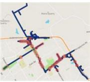
LiDAR view of a circuit showing vegetation encroachment
